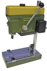
Ø1.00mm to Ø3.20mm Capacity - Proxxon TBM
