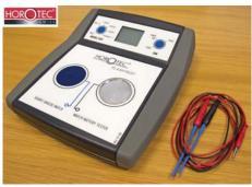
An all in one ergonomic device for complete testing of quartz watches & movements
