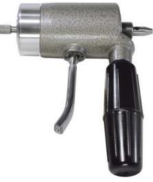
Hand polishing system developed for the watch industry, in particular watch cases. The arbour attaches to the vice and rests on a ball bearing. This means that as soon as the item being polished (held by the arbour) comes into contact with the polishing wheel, the item spins at the same speed as the wheel.
