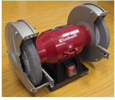
This quality bench grinder is perfect for all engraving tool shaping requirements. Gravers come in a standard size and length so they have to be grinded down to specific hand size and shape.
