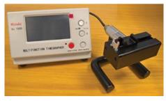
New watch timing & testing equipment for mechanical watches
