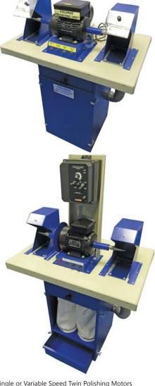
Single or Variable Speed Twin Polishing Motors
