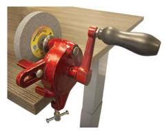
This manual bench grinder is perfect for all engraving tool shaping requirements. Gravers come in a standard size and length so they have to be grinded down to specific hand size and shape.
